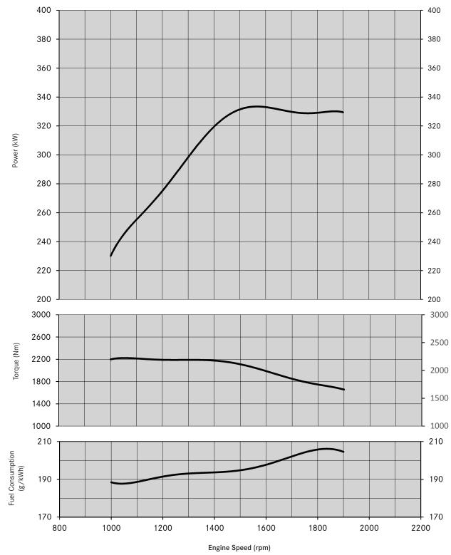
**Power, Torque** OM 460, 330 kW at 1600/min, Euro III 2200Nm at 1100/min
