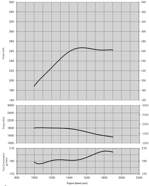
**Power, Torque** OM 440, 265 KW at 1600/min, Euro III 2600Nm at 1100/min
