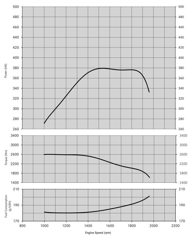
Power, Torque OM 473, 380 kW at 1600/min, Euro III 2600Nm at 1100/min
