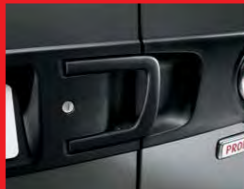
Rear wing door handle which is easy to open, even with a single finger
